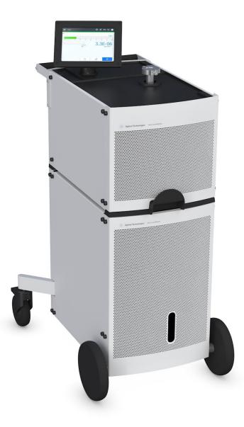
Improved power-off process, keeps spectrometer under vacuum and protects turbomolecular pump
